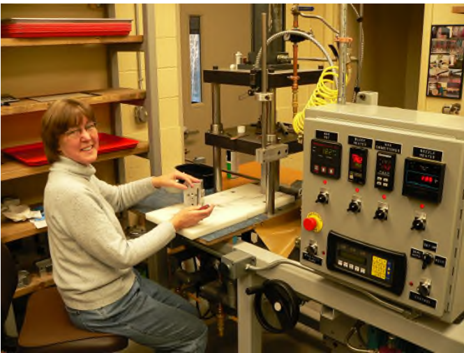
Janice uses the continuous wax injector to create the wax patterns. The patterns are assembled on to trees that are later surrounded by the investment.
