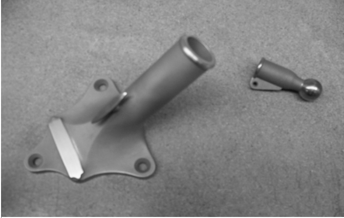
A flag holder and flag pole tip designed by John and Janice Hildebran. The buffed nameplate is ready for engraving.
