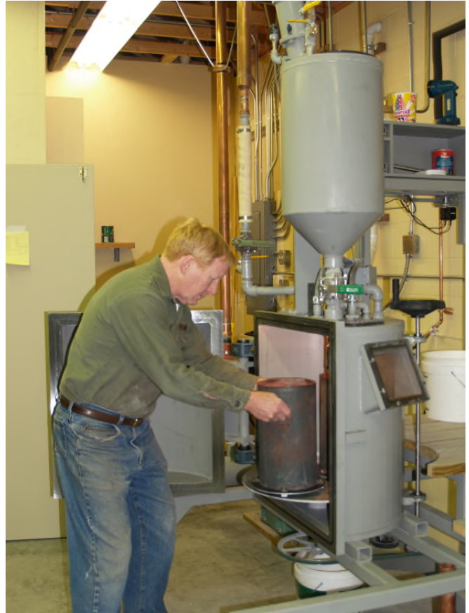
John places a flask with a pattern tree set inside it, into one of many, custom Hildebran designed and built machines. This unit mixes and injects the investment ( a unique type of plaster) into the flask. This entire process is accomplished in a vacuum chamber which eliminates any bubbles forming on the surface of the parts and ruining them. The investment hardens in 20 minutes and is ready for the next phase. In the shell molding process this process could take as long as 3 days.
