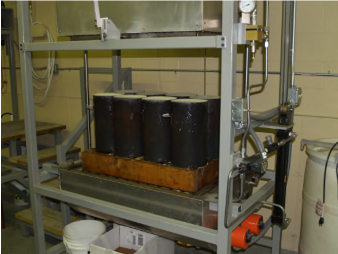
Next, the filled flasks are ready for de-waxing. With the wax removed, the empty void leaves the investment with a reversed negative of the parts to be poured, creating a perfect, highly detailed part.
